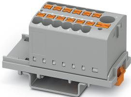
Distribution block, Block with vertical alignment and integrated supply, the blocks can be bridged with one another via the conductor shaft, for corresponding plug-in bridges, see accessories, nom. voltage: 690 V, nominal current: 24 A, connection method: Push-in connection, Push-in connection, number of connections: 13, cross section: 0.14 mm<sup>2</sup> - 4 mm<sup>2</sup>, AWG: 26 - 12, width: 28.6 mm, color: gray, mounting type: NS 35/7,5, NS 35/15
